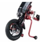
LED light, Carbon fender, discbrake
